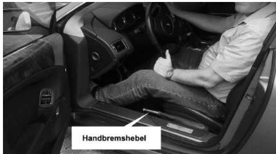
Рис. 25. Figure: Handbrake lever (Handbremshebel) on localized English car for LH drive markets
